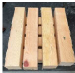
Placement of the fuel load in the firebox
