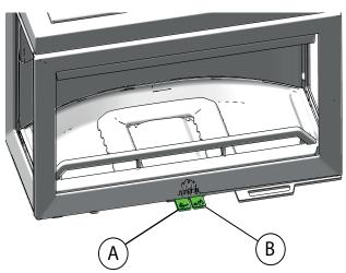
Pull out the ignition vent (A) (the air vent (B) follows automatically).
