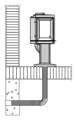
Fig. 3d Indirectly through an outside wall
