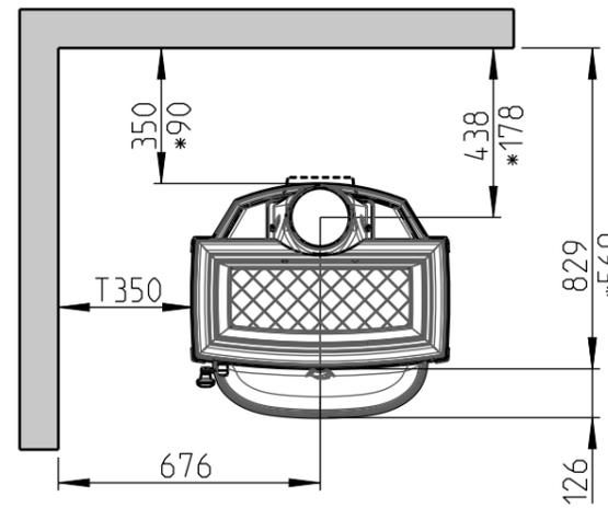
\* With semi-insulated flue pipe and extra heatshield
