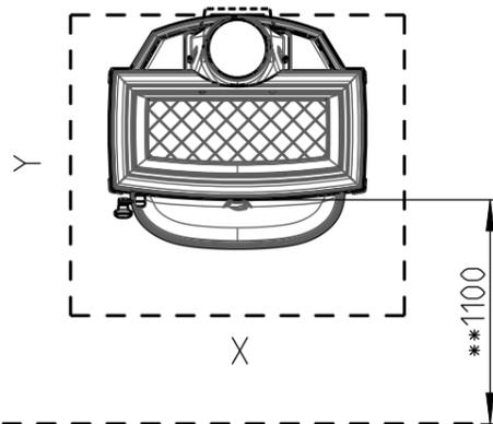
Min. measurements floor plate
